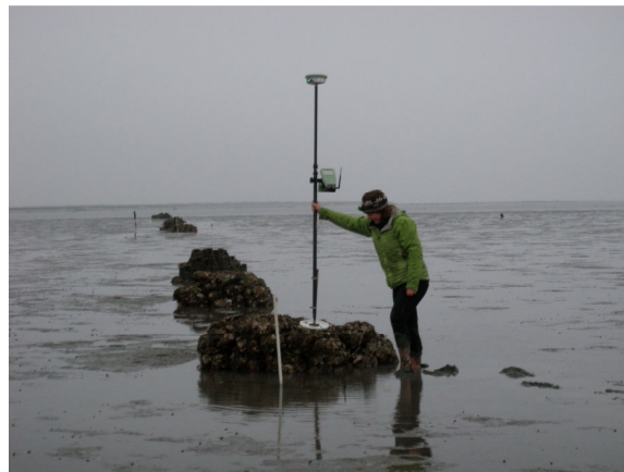
Figure 5. RTK-GPS survey of element elevation
